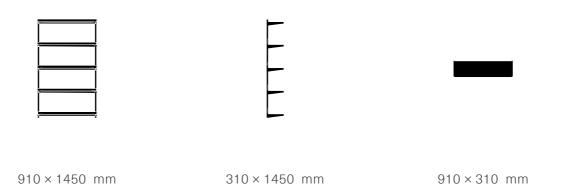
CLICK is a boltless shelving system. The minimalistic form and construction, as well as the visual lightness, form the aesthetic characteristics of the shelf. Constructed of 2.5mm thin sheet steel, a girder and shelves, the system functions similar to a construction kit. Only four screws fix the girder together to which the shelves are simply hung up without any tools. The material and precision of the components guarantee the stability and assembly.
